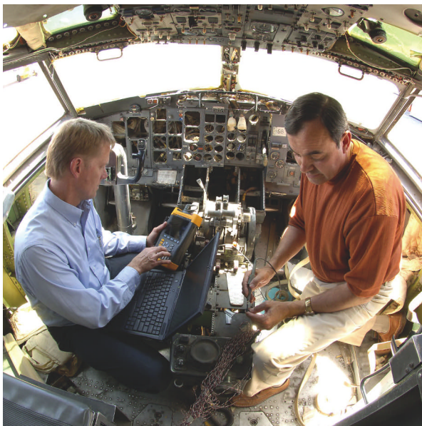
Researchers prepare to test the condition of a wiring bundle in the cockpit of a retired Boeing 737.
